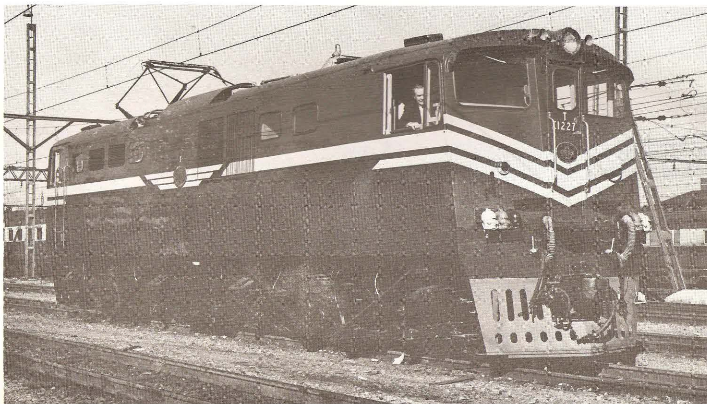
South African Railways Class 6E1 electric locomotive of 2,500 kW
